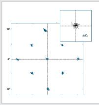
support using the Remote Camera Upgrade. Repeated target fixations to nine screen locations resulted in the low error levels demonstrated by the fixation error histogram below (Mean = 0.41°, Median = 0.40° and Standard Deviation = 0.22°). The inset plot is an enlarged view of the fixation distribution around the center target position. See Page 4 for analogous data using head-stabilized tracking.
