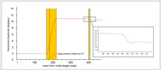
The EyeLink 1000 Plus has outstanding real-time data access to high-resolution data. Here, the participant made a saccade to a peripheral target that was moved by 0.8° about 21 msec after the saccade was initiated. A 0.33° corrective saccade lasting 8 msec occurred in the direction of the target position change.
