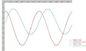
The Portable Duo produces stable, low-noise, binocular recordings, even when the head is freely moving (at up to 1000 Hz, and up to 2000 Hz with the head stabilized). In the above remote, head free-to-move eye traces, small corrective saccades can clearly be seen in the binocular circular smooth pursuit data.
