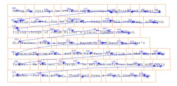
Sample reading data showing interest areas automatically generated by the Experiment Builder software, with eye traces and fixations overlaid using EyeLink Data Viewer.
