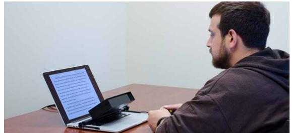
The EyeLink Portable Duo includes adjustable Tripod and Laptop Mounts to enable superior quality eye tracking data collection in a wide variety of settings, both in and out of the laboratory.
