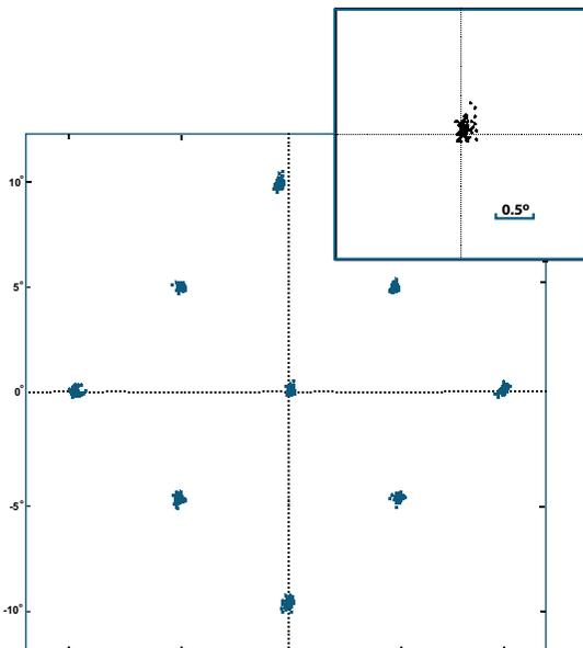
Accuracy was assessed without a head support using the Remote Mode following a 13-point calibration. Repeated target fixations to nine screen locations resulted in the low error levels demonstrated by the fixation error histogram below (Mean =  $0.26^\circ$ , Median =  $0.22^\circ$  and Standard Deviation =  $0.16^\circ$ ). The inset plot is an enlarged view of the fixation distribution around the center target position.
