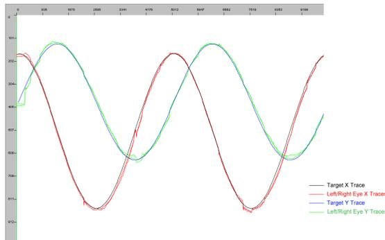
The Portable Duo produces stable, low-noise, binocular recordings, even when the head is freely moving (at up to 1000 Hz, and up to 2000 Hz with the head stabilized). In the above remote, head free-to-move eye traces, small corrective saccades can clearly be seen in the binocular circular smooth pursuit data.
