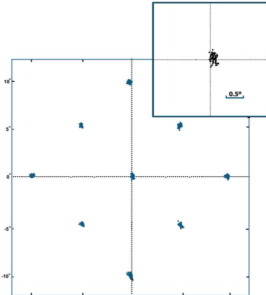
Repeated target fixations to nine screen locations recorded with the EyeLink Portable Duo with the head stabilized following a 13-point calibration. The inset plot represents an enlarged view of the fixation distribution around the center target position. On the right is a fixation error histogram demonstrating the tight fixation accuracy distribution (Mean =  $0.25^\circ$ , Median =  $0.23^\circ$ , and Standard Deviation =  $0.14^\circ$ ).
