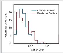
Repeated target fixations to nine screen locations recorded with the EyeLink 1000 Plus with the head stabilized. The inset plot represents an enlarged view of the fixation distribution around the center target position. On the right is a fixation error histogram demonstrating the tight fixation accuracy distribution (Mean = 0.33°, Median = 0.29°, and Standard Deviation = 0.20°).
