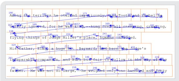
Reading data showing interest areas automatically generated by Experiment Builder software, with eye traces and fixations overlaid using EyeLink Data Viewer.
