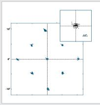
fixations to nine screen locations resulted in the low error levels demonstrated by the fixation error histogram below (Mean = 0.41°, Median = 0.40° and Standard Deviation = 0.22°). The inset plot is an enlarged view of the fixation distribution around the center target position. See Page 4 for analogous data using head-stabilized tracking.
