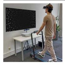
When combined with a treadmill, the EyeLink 3 is a convenient tool for research into combined eye and head movements during gait. It can also be combined with a balance / force place for research into the role of head and eye movements in balance.
