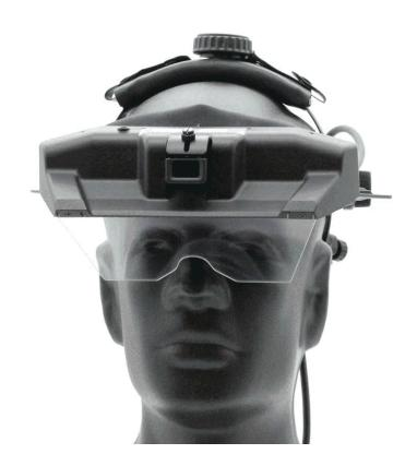
SR Research introduces the <u>EyeLink 3</u>, an advanced head and eye tracker for screen-based research. It records synchronized head and eye data at up to 1000 Hz, offers full <u>six-degrees of freedom head-tracking</u> and provides novel pixel-based <u>eye and head position data</u>, along with typical gaze data. The EyeLink 3 also records high-speed (up to 500 fps) eye video, opening up new possibilities for exploring perceptual and cognitive processes in a more natural context.
